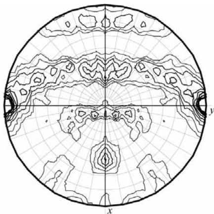
Figure 2 Representation of the \chi = 180^\circ section of the self-rotation function of PaGS crystals. The orthogonalization code follows the PDB convention. See text for interpretation.
